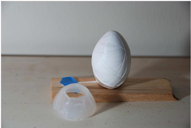
Illustration 12: Retainer and Wooden Egg Covered with Teflon Tape
