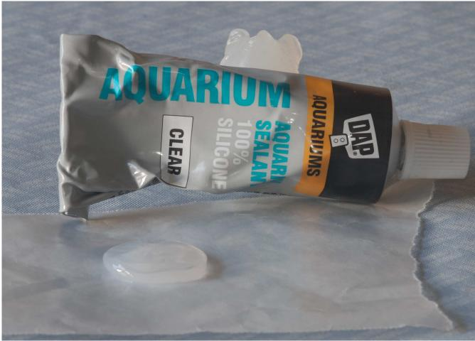
Illustration 1: Silicon Disk Ready to be used as a Small Insert
